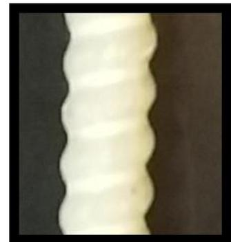
**FRP threaded rods and nuts. 18mm diameter.**
